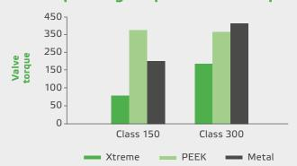
Operating torque and required actuator size is much lower than PEEK or metal seats.
