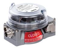
The Axiom<sup>™</sup> provides advanced monitoring and control in explosionproof, non-incendive, intrinsically safe and general-purpose applications. It is a discrete on/off valve controller with proximity switches for quarter-turn automated valves. Its rugged construction will withstand the most challenging plant environments.
