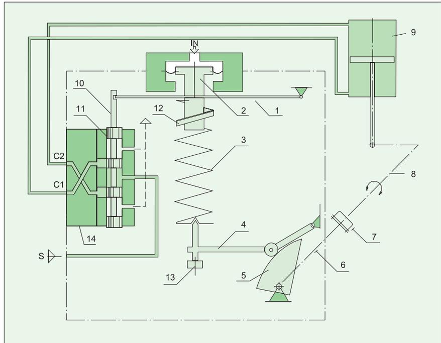
Operation is based on the force balance principle. One force is caused by signal pressure (IN) transmitted through the diaphragm (2), the other force is caused by the feedback spring (3). The latter is directly proportional to the position of the lower end of the spring, this in turn depends solely on the actuator shaft (8) position as transmitted through the coupling (7), shaft (6), cam (5), and the lever (4). When these forces are not equal, the beam (1) moves in the direction of
